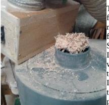
The DUST collector found its match recently when it filledup with SHAVINGS. I suspect the planer was being used at too high a setting. It took several goes to clean out the pipe.
