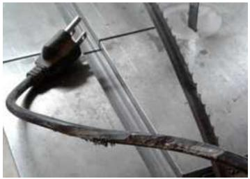
If you can't see the **BARE WIRES**, go get your glasses! This was the power cable for the small band saw, it had been rubbing on the side of the **belt sander**. There is a hook on the post to hold the wire away from such, please make sure that's where it's at.
