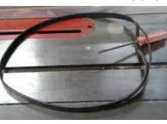
The **Table Saw** was making aweful noises the other day and on opening the belt cover I found the multi-V belt was running on the motor shaft and the pulley was pushed up
