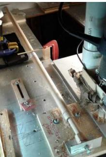
and just need to shape the end accordingly. Here you see the top with a tonge to fit up into the head and a 15/16"dia section tor the self threading collar. At least that's what the Lee Valley Tools instuctions said but they're a bit out of wack! For the tip I added a 3/4" round with a 20" taper. The CNC won't actually rotate the job so that was done by hand with cuts being made
