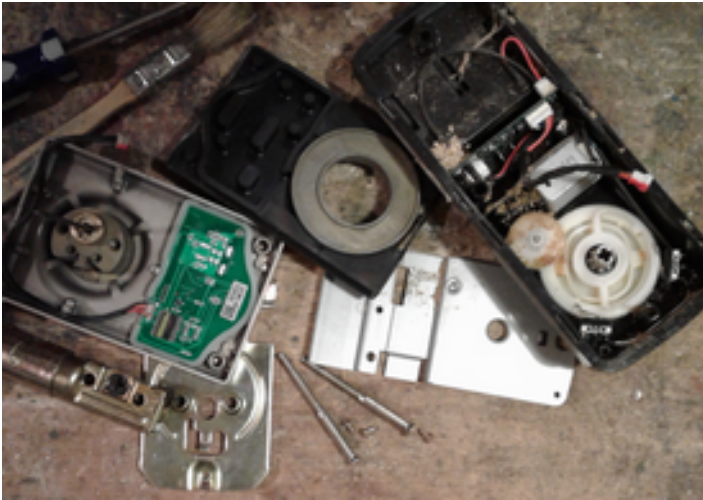
We've taken the old door lock to pieces and discovered an ants sawdust pantry inside, right over the motors plastic worm gear. Of course this and the small round gear are well greased so it made for a sticky mess and likely slowed things down a bit.
