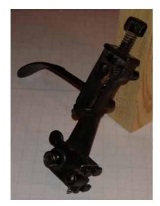
This assembly is strong enough to clamp an oscillating blade but still deserves a bit of care and adjustment. A thicker blade might need the lower bolt to be opened to move the clamping jaws out a hair. The small spring came from my workshop's 'stock', while the clip was fabricated from a short length of spring wire. The drawing below shows the approximate dimensions should the occasion arise!
