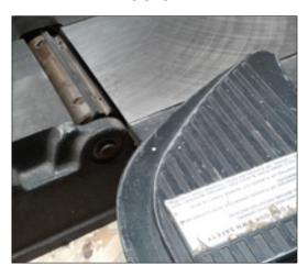
Geoff, with some help from Ross, recently replaced the Jointer blades. In doing so they found the body of the beast packed with shavings. It had likely been run without the Dust collector functioning. There is a plethora of gates on the ducts behind which require opening and closing in some semblance of order. A single screw will remove the pipe underneath. Unless you are looking for a manicure please disconnect the Jointer POWER before delving any further.
