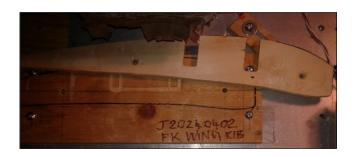
The shelves above the Table Saw can now be used to hold Jigs and the like. You won't find this one as it's intended for the CNC machine. It holds a Fokker rib for cutting out the 3/4" strut notches. You'll notice each rib has two 1/4" alignment bolt holes and so does the jig. Once the CNC set-up is complete it becomes 'bolt down and hit GO'... when it works!.
