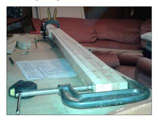
Each strut and edge also requires 3/8" grooves which can be done at the shed using a router (red handled) and yet another Jig.
