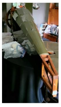
**Fokker DR1 Fuselage:** Another day another strip. Each outside runner is made up of 9 1/4" square strips. On this lower aft section they curve both in and up. Cross pieces are temporarily nailed to the jig walls. Clamps and clamps and plastic pegs...
