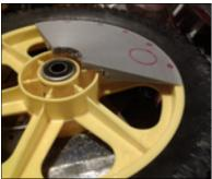
undercarriage. They each have a pair of 1/2" bearings and a removal hubcap.
