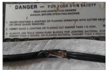
Don't ask what took me behind our Jointer but here is what I found. The green Ground wire is eaten halfway through, the white Neutral is opened up and the black Live is being worked on. The cable was sat on the belt having been pushed there by the dust pipe. The belt does not have a cover, the cable was not secured. The cable ran between the wall outlet and the Jointer switch, it was very much **alive**.
