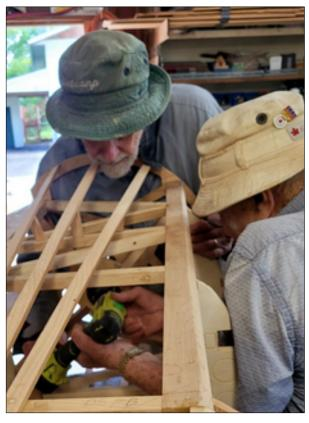
Fokker DR1 - Paul and Dave trying to install the gas pipe engine shaft between a hole in the firewall and a pipe socket on the Engine Brace. It was a tight spot to wield the drill with one trying to support the battery while t'other pushed and kept it aligned. Only three more screws to go.
