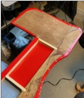
On the left is a thin aileron from the upper wings, partly covered by **John F.** The end section wraps around the wing tip so has yet to be shaped. John says he spends a lot of time on the wavey trailing edge.
