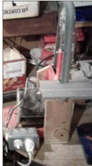
This home-workshop belt sander from Lee Valley did not come with a dust attachment so a wooden box was built for it to sit in. The original design had a pipe coming out of the front but this started to get in the way and was moved to the rear with the original hole bunged up with a wheel! The switch on the LHS turns on the sander but also powers the socket which runs a small vacuum tucked under the bench. DW
